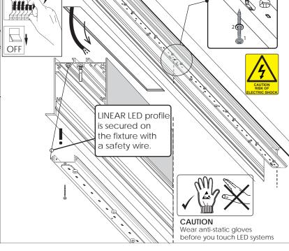
Access profile and make wiring connections.
