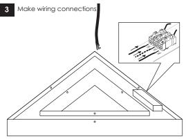
Fit the fixture on ceiling. Tighten the (6) screws.
