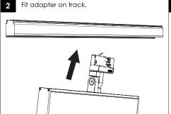
Push the adapter into track till it snaps into place. Turn the mechanical fixing knob. Select the deisired circuit.
