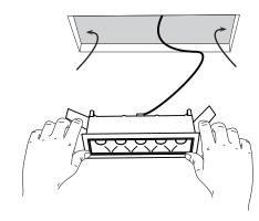
Fit the luminaire in the ceiling.
