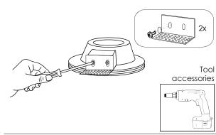
Screw the fixture on ceiling Hold the luminaire while using the drill.
