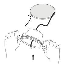
After installing the fitting, fill the gaps on ceiling. Then paint the ceiling.
